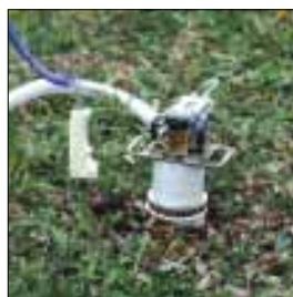
Figure 2. LI-6400 soil CO 2 flux system setup. The plumbing circuit highlighted in color is for CO 2 scrub operations; it is only used during the draw down portion of a measurement cycle. During the measurement, mixing in the chamber headspace is achieved with the gas analyzer mixing fan and manifold.
