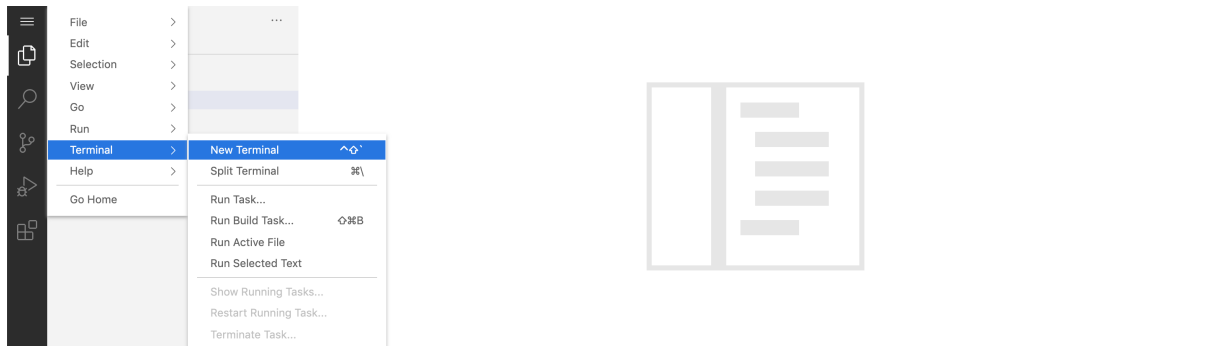
Figure 1.1: You can open a new terminal by clicking on the burger icon ( \equiv ) and then navigating to “Terminal -> New Terminal”.
