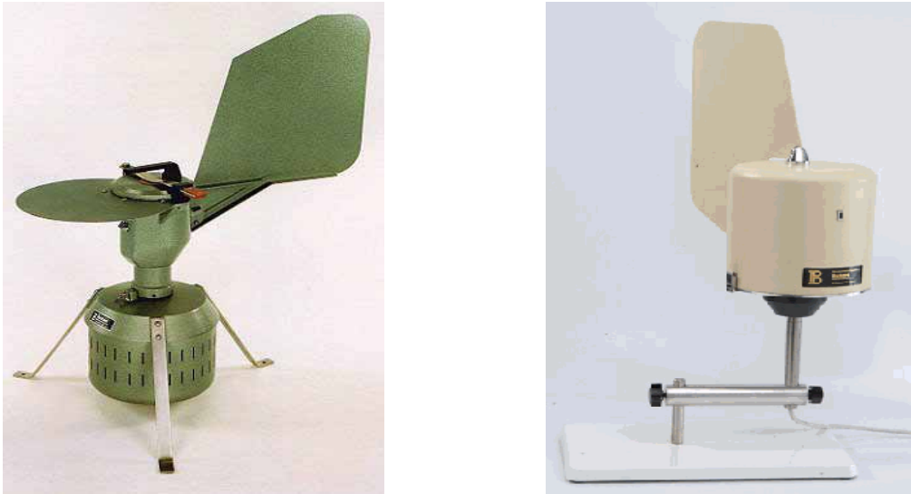
Figure 3. Types of spore traps used in the SPEC project: left: seven-day volumetric spore trap, right: multi-vial cyclone spore sampler (Burkard Manufacturing Inc.)
