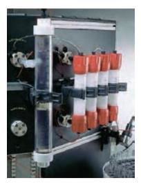
Fig 2.6. A 60 ml sample volume can be run on four HiPrep 26/10 Desalting columns connected in series.
