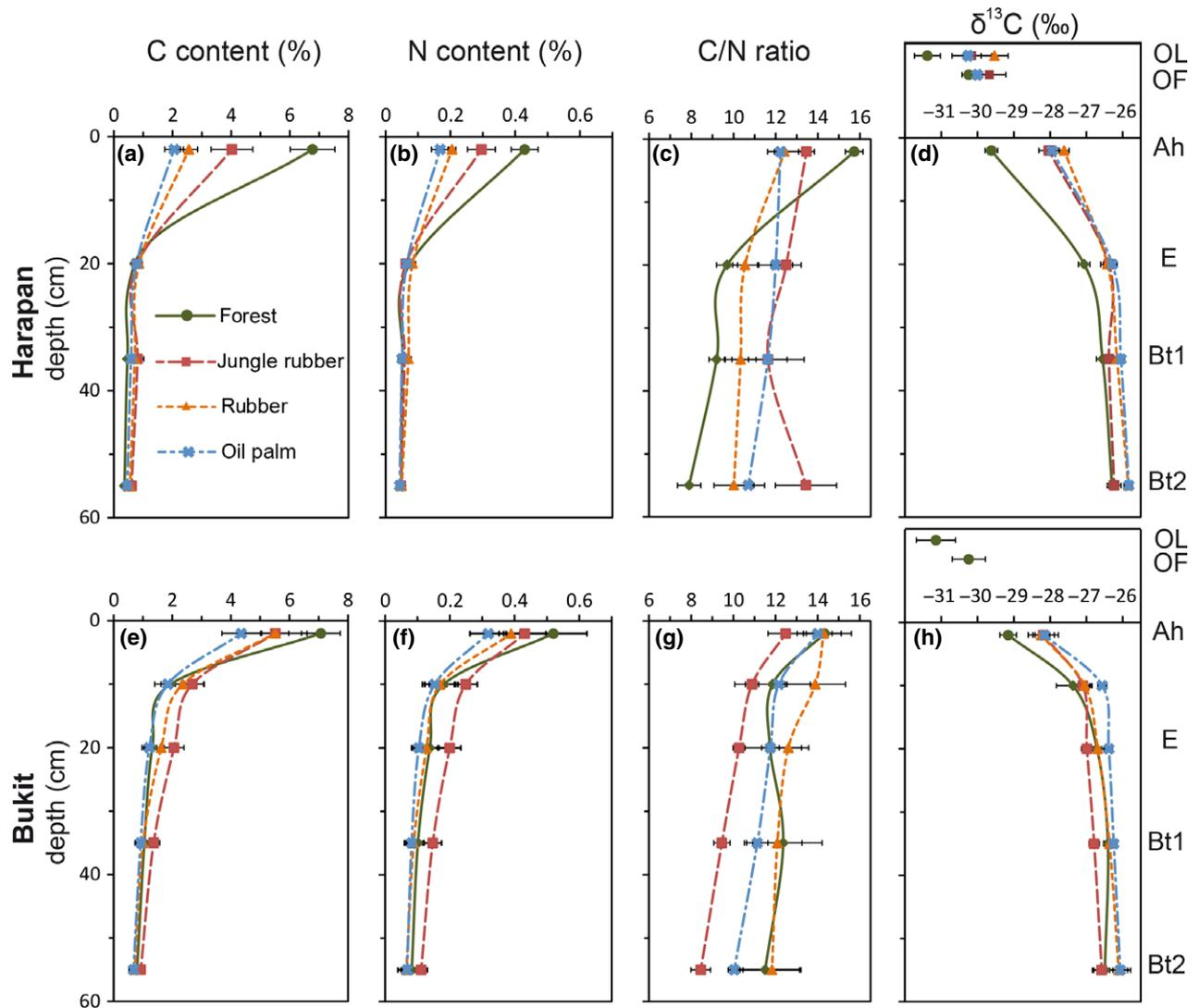
**Fig. 3** Soil characteristics distributions with soil depth. (a,e) Carbon content, (b,f) nitrogen content, (c,g) C/N ratio, and (d,h)  $\delta^{13}\text{C}$  distributions under forest, jungle rubber, rubber, and oil palm plantations in (a–d) Harapan and (e–h) Bukit regions. Values at fixed depths were recalculated from the original sampling points, except for Ah horizons. Ah horizon depth fixed at 1 cm for presentation purpose. Values represent means  $\pm$  SE ( $n = 4$ ).
