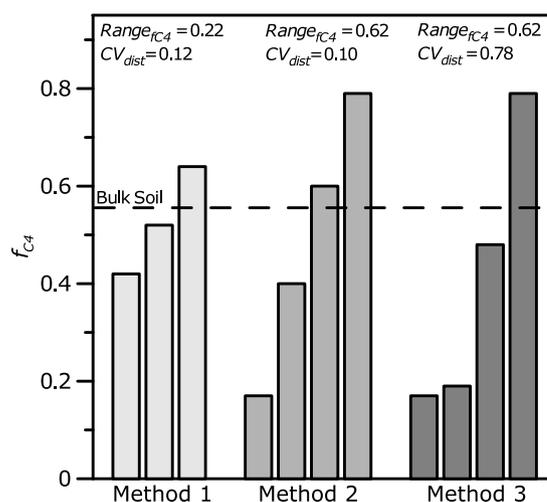
Fig. 1. Example of three soil fractionation methods (methods 1–3) with varying ranges of  $f_{C4}$  between soil fractions (indicator for differentiation of turnover rates) and varying  $\text{CV}_{\text{dist}}$  (indicator of redundancy in turnover rates). Each bar represents one fraction.
