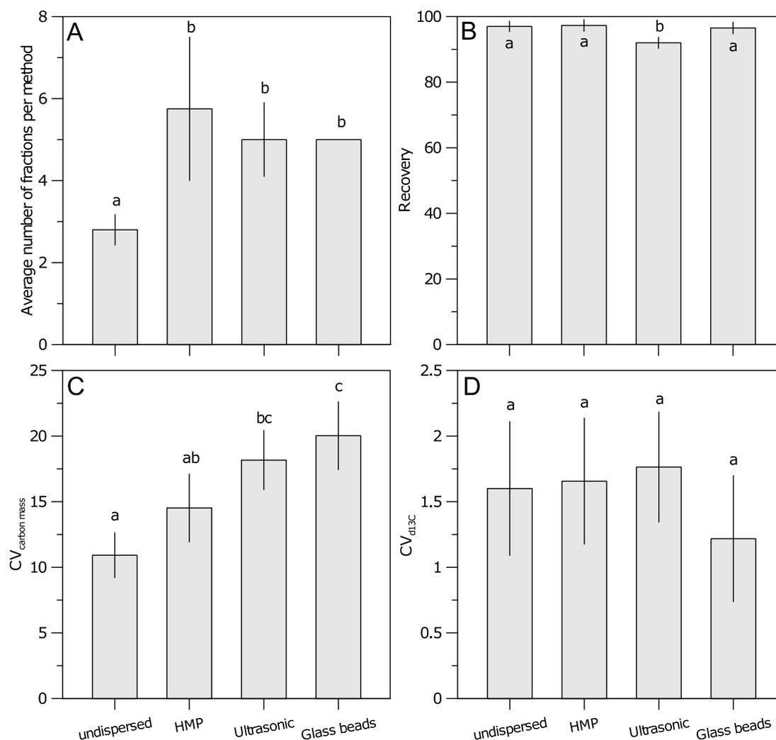
**Fig. 8.** A) Average number of fractions per method, B) average recovery [%], C) average coefficient of variation of carbon mass across replicates, D) average coefficient of variation of  $\delta^{13}\text{C}$  values across replicates for different soil dispersion methods. Error bars indicate standard errors and different letters indicate significant differences.
