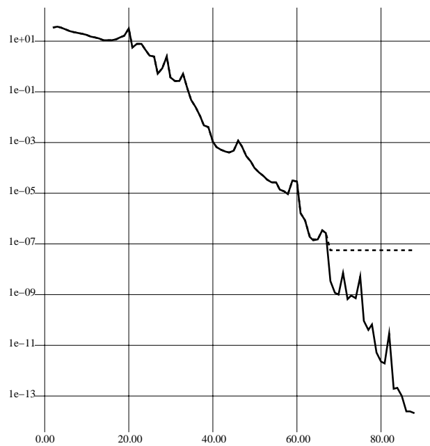
Figure 4: Updated (solid line) and true (dashed line) residual for BiCGstab without search directions on model problem (16)
